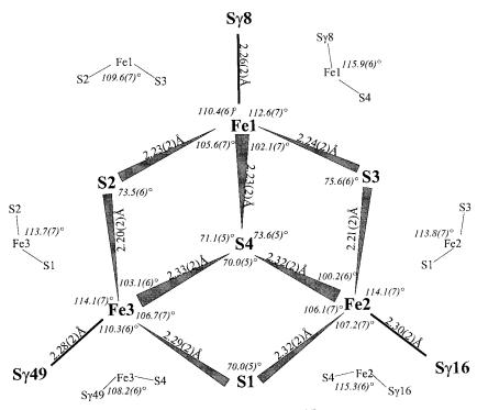
FIGURE 3: Schematic diagram of the structure and atom labeling for the  $[3Fe-4S]^{+/0}$  cluster in FdI with bond lengths, angles, and *su* values determined for the Red1 structure (Tables 3, 4).
